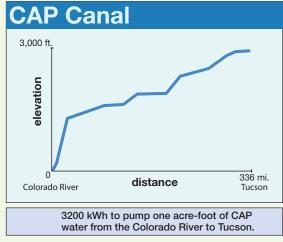
Interbasin water transfers in Arizona and Nogales, Sonora require large amounts of energy. The profile of the Central Arizona Project through Arizona (right) shows an increase in elevation of 2900 feet from the Colorado River to its end near Tucson. The Los Alisos/Rio Magdalena-Nogales aqueduct in northern Sonora must cross over a watershed divide to reach Nogales.
